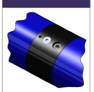
Mechanical activation indicator built into the tool which can be re-set at surface.
